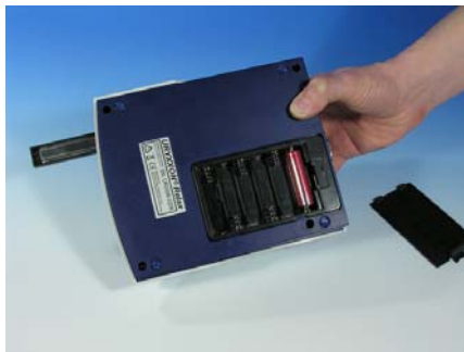
Pic. 3.10 : battery compartment
