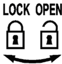
Figure 4-6 Lock and Open Marks on Probe Connectors
