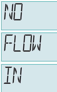
Figure 3-4 NO FLOW IN Alarm
