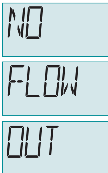
Figure 3-5 NO FLOW OUT Alarm
